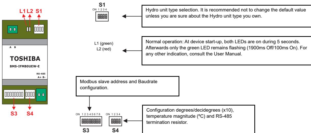
The following table applies for configuration of the interface through these DIP-switches:
