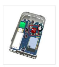
To access the built-in DIP Switch block, open the enclosure by releasing the rear lid. Next, gently bend both frontal click-fit tabs by inserting a flat-tipped tool (size < 5 mm). This operation must be performed by qualified personnel only.
