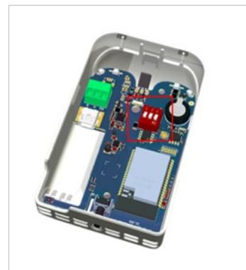
To access the built-in DIP Switch block, open the enclosure by releasing the rear lid. Next, gently bend both frontal click-fit tabs by inserting a flat-tipped tool (size < 5 mm). This operation must be performed by qualified personnel only.
