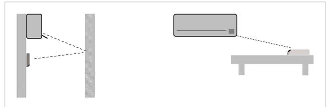
Placing the device under the AC unit (left) or on a desktop (right)
