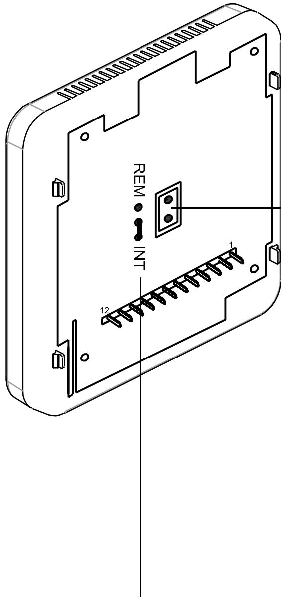
**ITA** CONNETTORE SENSORE ARIA ESTERNO**ENG** EXTERNAL AIR SENSOR CONNECTOR**FRA** CONNECTEUR CAPTEUR D'AIR EXTERNE**DEU** ANSCHLUSS FÜR DEN AUSSENLUFTSENSOR**ESP** CONECTOR DEL SENSOR DE AIRE EXTERNO**RUS** РАЗЪЕМ ВНЕШНЕГО ДАТЧИКА ВОЗДУХА
