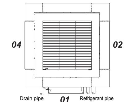
**3 Determine wind direction of the selected louver by pushing SWING/FIX.**
