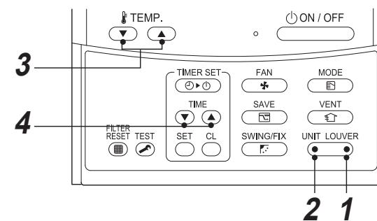
**1** Push **UNIT LOUVER** (right side of the button) for at least four seconds when the air conditioner is not working.
