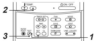
1 When **SET** and **TEST** buttons are pushed at the same time for 4 seconds or more, the following display appears.
