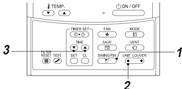
**1** Push **SWING/FIX** for at least four seconds when the air conditioner is not working.
