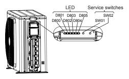
3. Turn on the circuit breaker to supply electricity.
