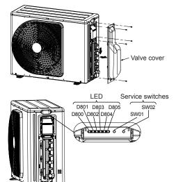
3. Turn on the circuit breaker to supply electricity. In the initial LED display status, D805 is lighted as below.
