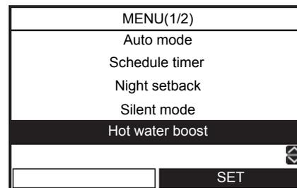
(2) Press the [ ▲ ] button to select "ON" on the Hot water boost screen, then press the [ FIX ] button. The
