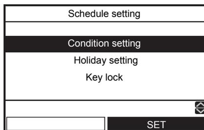
(2) Press the [ F1 ] button to select the day, then press the [ F2 ] button to input running pattern.
